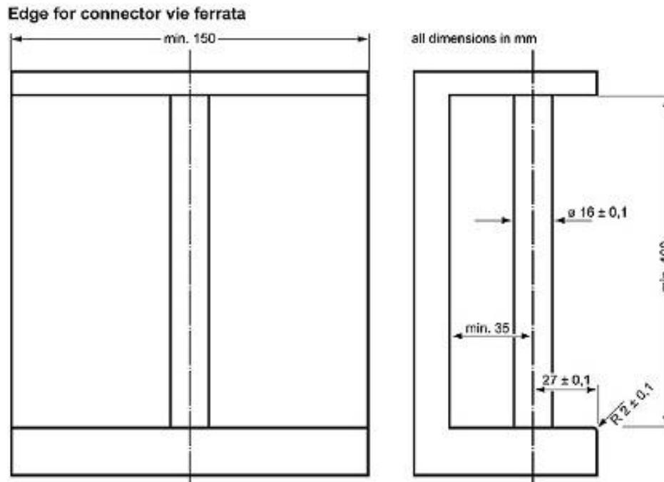
**Figure 1 Test Edge for type K connectors**
