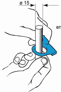
The eye shall be large enough that a bolt as shown can be inserted
