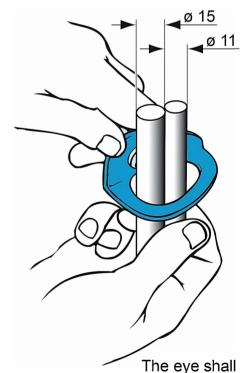
be large enough that two bolts as shown can be inserted
