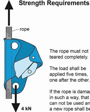
The rope must not be teared completely.
