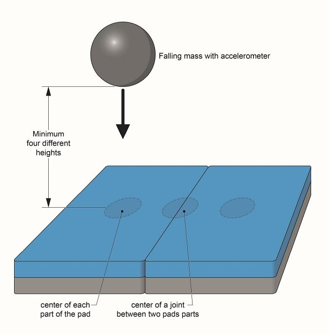
The lowest drop height producing a Head Injury Criterion (HIC) value of 400 determines the critical fall height.
