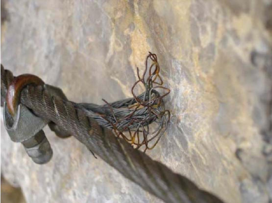
**Fig 27** Defective cable
