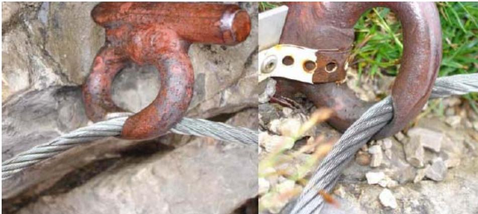
**Fig 18** Friction wear of eyebolts.
