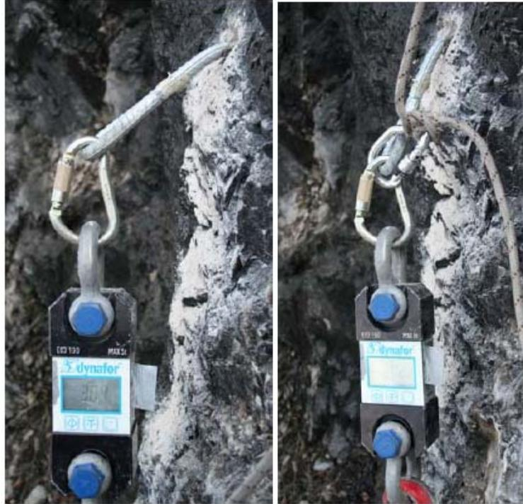
**Fig 12** Bending due to 3 kN and 6 kN
