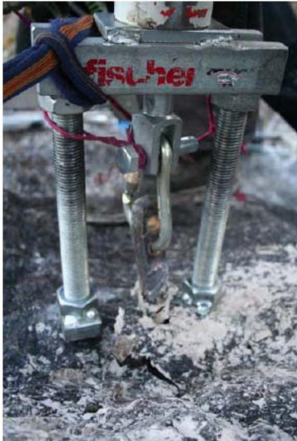
**Fig 14** Axial pull of an anchor with the tensile tester
