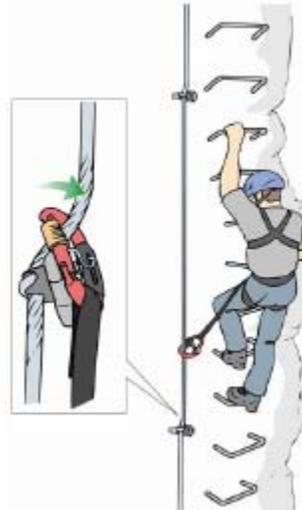
**Fig 5** Eastern alps/classical system with tensioned or untensioned cable through eyebolts, possibly clamped
