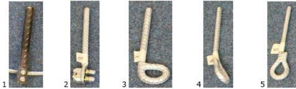
1 32 mm U-clamp anchor 2 20 mm U-clamp anchor 3 20 mm eyebolt (mfr. Schiestl) 4 16 mm angled eyebolt 5 16 mm eyebolt
