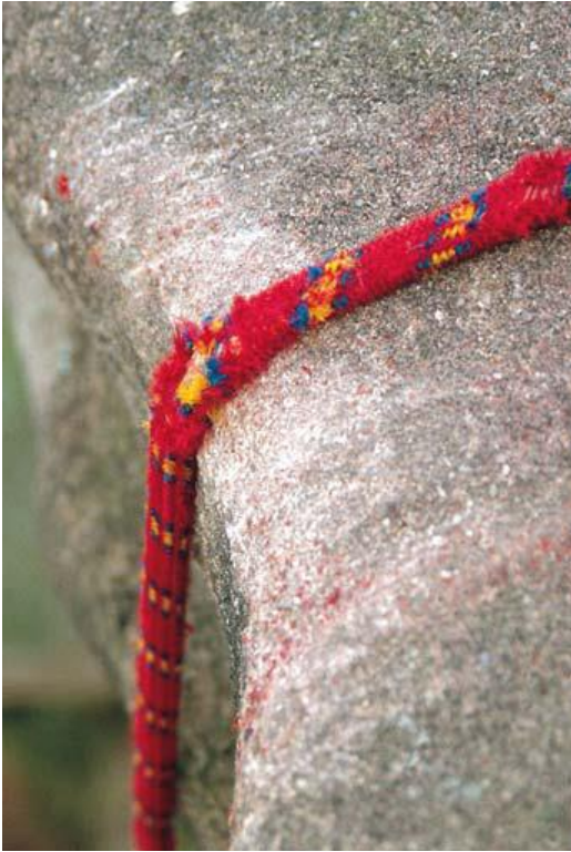
Figure 10.3 Serious damage to a rope in use Photo: BMC Collection
