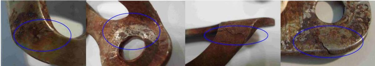
**4- Examples of weakened anchors with No visible cracks, but which broke between 1 and 5 KN:**
