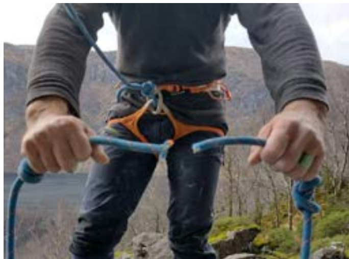
Rope cut by falling rocks at the Hetta climbing crag in Vaksdal. The picture above shows the cut rope. The picture below shows the rock that came loose when the climber stepped on it.
